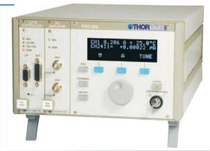
The PRO800, chassis accepts two 8000 series modules. Use our LDC8000 and our TED8000 series modules to set up a space saving laser current & temperature controller...
